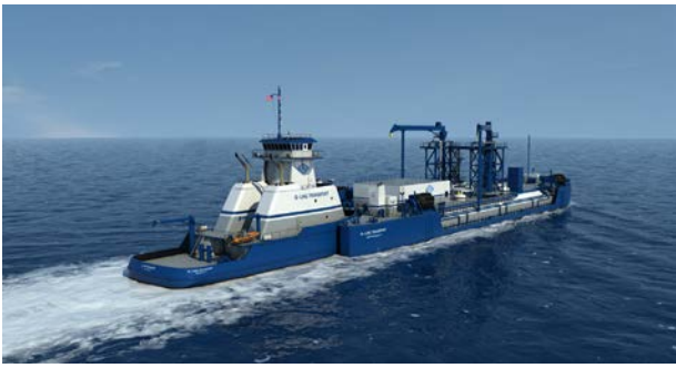
Figure 5. Q-LNG Transport LNG Articulated Tug and Barge (courtesy of Harvey Gulf International Marine).
