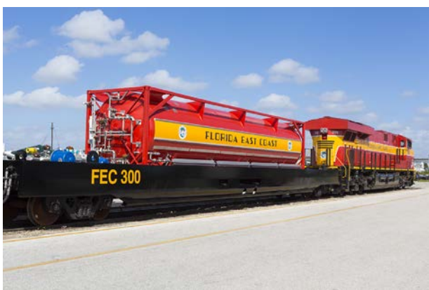
Figure 2. FEC Railway LNG fuel tender and locomotive (courtesy of Florida East Coast Railway).
