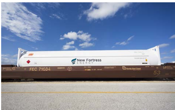
Figure 3. New Fortress Energy LNG ISO container (courtesy of Florida East Coast Railroad).
