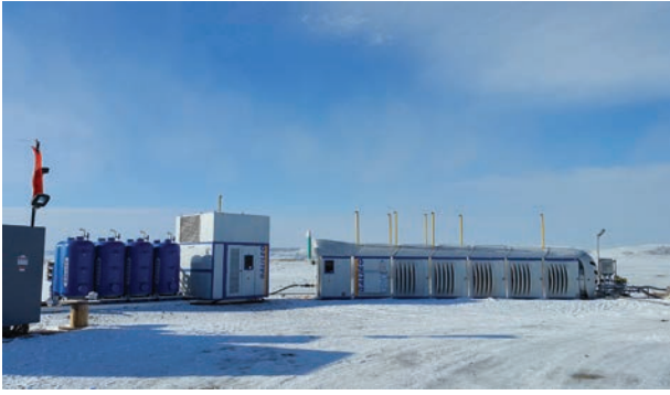
Figure 7. Galileo Cryobox® installation in the Bakken for flare gas reduction (courtesy of Galileo Technologies).
