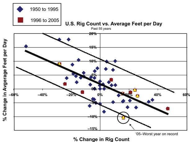
Fig. 5—Rig-count/drilling-performance correlation.
